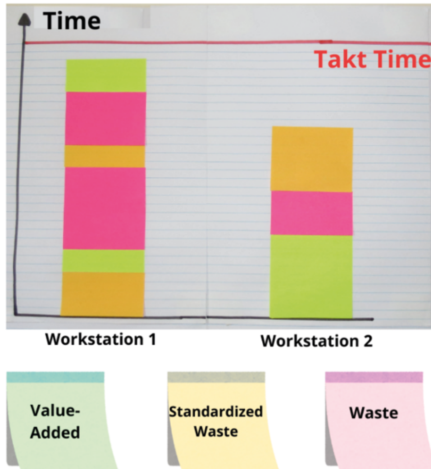
Figure 8.9 – Yamazumi built with Post-its
